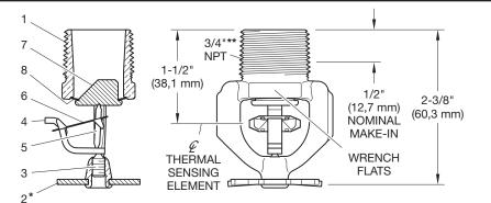
FIGURE 1 MODEL ESFR-17 PENDENT SPRINKLER, 16.8K, 165°F (74°C) EARLY SUPPRESSION, FAST RESPONSE
